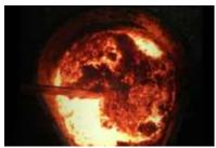
When melted the worthless rock becomes separated from the gold and can be scraped away
