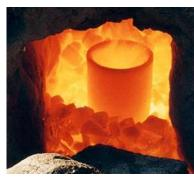
The rock is placed in a container called a crucible and put into the hot furnace
